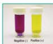
YCA-106A Yeast Acid Food Medium Product Specifications Testing time: 4-72 hours Tests per kit: 100
